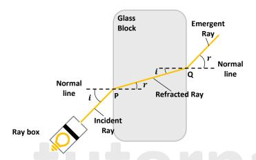
Note: The angle of incidence, i is the angle formed by the incident light ray and the normal.
