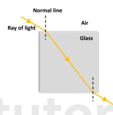
Consider the diagram above, which shows how a light ray changes direction as it enters and exits a rectangular glass block in air. When the light ray travels:
