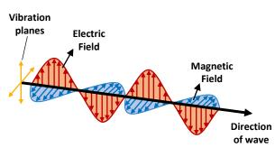
A wave that is unpolarised has vibrations in all directions that are at right angle to the wave's direction.
