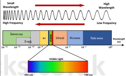
The wave properties become more obvious as the wavelength increases - for example, long radio waves can diffract around hills whereas visible light can only diffract through a very narrow slit.
