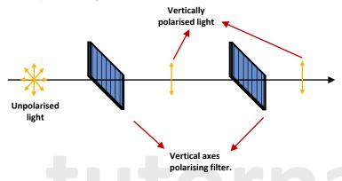
Less and less light is transmitted as the second polaroid is progressively rotated such that its polarisation axis moves from vertical to horizontal. When the axes of the two polaroid's are at right angles to one another, no light is transferred.
