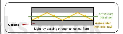
**Material dispersion:** is caused by the different amounts of refraction experienced by different wavelengths of light. Different wavelengths slow down by different amounts in a material. Since light is made up of many different wavelengths, some parts of the signal take longer to travel down the fibre than others. Material dispersion can be prevented by using monochromatic light.
