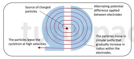
Charged particles are created and shot in all directions from the source into one of the electrodes, where they follow an oval/circular path and eventually exit the electrode due to the magnetic field. An applied p.d. between the electrodes accelerate the particles across the gap until they enter the next electrode.
