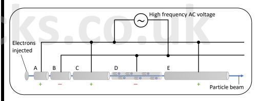
The alternating voltage supply is made to change as the electrons reach the centre of tube A. So, tube A will be positive at first pulling in the electron. As soon as the electrons reach the halfway point, tube A becomes negative which repels the electrons out of the end of tube A. But while tube A is now negative, tube B becomes positive. This not only draws the electrons as they exit tube A, but it also causes them to accelerate toward tube B.
