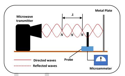
Microwaves can be directed towards a metal plate using a microwave transmitter attached to a signal generator, as seen above. At the metal plate, the microwaves are reflected back to the emitter.
