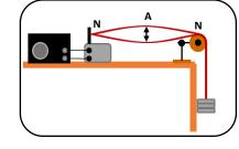
This stationary wave with a single loop at the fundamental mode of vibration can also be called the 1<sup>st</sup> Harmonic.
