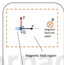
A moving electric charge enters a magnetic field at a 90° to the direction of the field's flux density (B).
