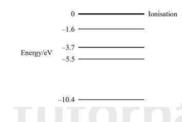
a) Calculate the ionisation energy in joules for an electron in the  $-10.4 \ eV$  level.
