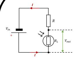
A light-dependent resistor (LDR) can be used in a potential divider to generate a variable output p.d.  $(V_{out})$  which varies with light intensity. This is illustrated in the diagram opposite.
