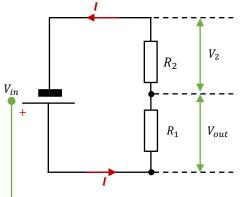
Consider two resistors  $R_1$  and  $R_2$ , which are connected in series to a source of fixed p.d.  $V_{in}$  as illustrated opposite.
