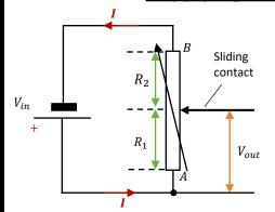
A variable resistor is used in the potential divider circuit opposite to produce a continuously variable output p.d. from a fixed input p.d.
