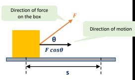
Movement only takes place in the horizontal direction in the diagram above. The vertical force does not cause any motion and hence isn't doing any work. The vertical force is only present to balance out some of the weight from the object and therefore the reaction force is smaller.
