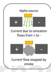
Smoke entering the chamber absorbs a-particles, reducing ionisation and thus the detected current. The electronic circuit detects the decrease in current and sounds the alarm.
