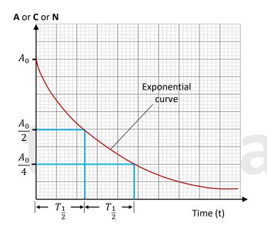
The graph shows how a radioactive sample's activity (A) or number of remaining unstable nuclei (N) decreases exponentially with time (t).
