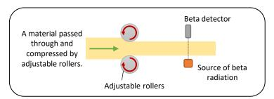
As the material passes through the rollers, it flattens out. On one side of the material, a radioactive source is installed, and on the other, a radioactive detector. The more radiation the material absorbs and stops from reaching the detector, the thicker it is. The rollers move closer together to make the material thinner if too much radiation is absorbed. They move further apart if not enough radiation is absorbed.
