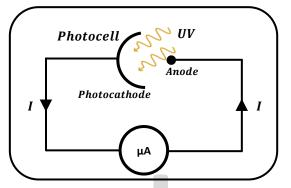
The photoelectric current, as measured by the microammeter, is proportional to the number of electrons flowing between the cathode and anode per second. Therefore, a high microammeter value indicates a high number of electrons released per second.
