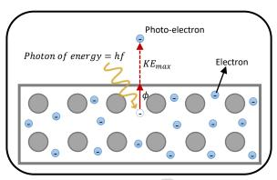
When a **photon of energy (hf)** causes photoemission from a metal surface, some of the photon energy is used to overcome the **work function** ( $\phi$ ), while the rest is released as kinetic energy.
