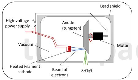
In an evacuated tube, a very high voltage ( $\approx 100 kV$ ) is applied across the electrodes (the cathode and the anode).
