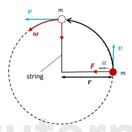
The centripetal acceleration (a) of an object of mass (m) travelling at a constant speed (v) in a circular path of radius (r) is given by:
