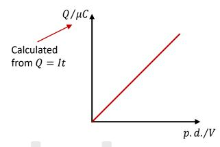
• The graph is a straight line through the origin therefore Q and V are directly proportional. The gradient of the graph is the capacitance, C, and so you can carry out the same experiment to calculate the unknown capacitance of a capacitor.
