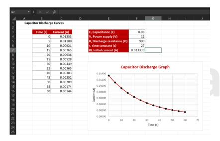
You can make the spreadsheet without any observation and experimentation. Using the mathematics we learnt about in this pack, provide the various cells formulae to calculate what capacitor theory tells us will happen,. The time constant cell (F6), for example, does not require user input because it is set to display the multiplication of the capacitance (F3) and discharge resistance (F5). This value is then used in the formula below for calculating the values in the "Current" column (C3),
