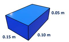
1) The only force that is being exerted on the surface of the desk is caused by the weight of the block. The weight force is acting perpendicularly to the desk:
