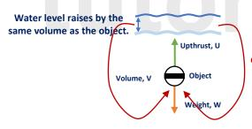
The displaced water doesn't like to be displaced so it will try to push down on the water around the object to push it back up.
