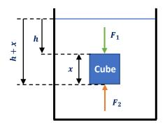
As  $P = \frac{F}{A}$  (where  $P = pressure\ due\ to\ the\ fluid\ and\ A = the\ cross - sectional\ area\ that\ the\ force\ acts\ on)$  we can rearrange to get force, F:
