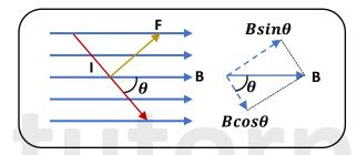
As a result, the force (F) acting on a wire of length (L) carrying a current (I) at an angle  $(\theta)$  to a uniform magnetic field of flux density (B) can be calculated using:
