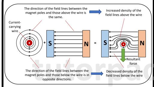
As a result when a current-carrying wire is placed in a uniform magnetic field between two magnet poles it will experience a resultant force.
