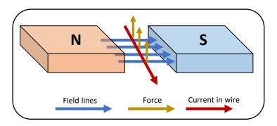
As indicated in the diagram above, a current-carrying wire placed in the magnetic field between two magnet poles experiences a force. The direction of current, magnetic field, and force are all perpendicular to one another.
