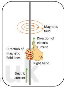
The direction of the magnetic field and current can be predicted using the: Right-Hand Grip Rule
