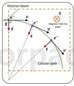
To use Fleming's LH rule for charged particles, use your second finger (current) as the direction of motion, but because electrons have a negative charge, an electron beam moving to the right is viewed as conventional current moving to the left. So point your second finger in the opposite direction to its motion. Thus the force (F) acting on an electron at point X is downwards, deflecting the beam in that direction.
