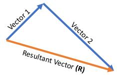
The <u>resultant</u> of a number of forces is the single force which has the <u>same effect</u>, in both magnitude and direction, as the <u>sum</u> of the individual forces.
