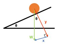
W = the weight of the object. The weight can be calculated using the formula:
