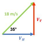
Vertical component  $(V_V)$ : Solve using trigonometry
