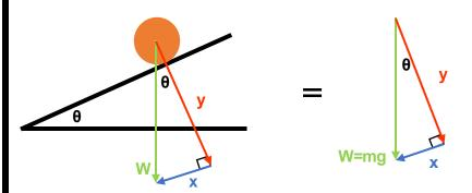
You can calculate the x and y components the same way you calculated the vertical and horizontal components of velocity in the previous examples. As you can see it's a right-angle triangle, so knowing that information you can use trigonometric functions:
