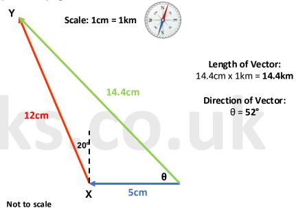
Displacement = 14.4 km with an angle of 52°
