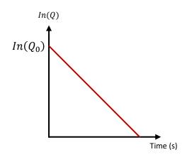
Because V and I have the same dependence on R and C, you could plot In(V) or In(I) against time and find the time constant in the same way.
