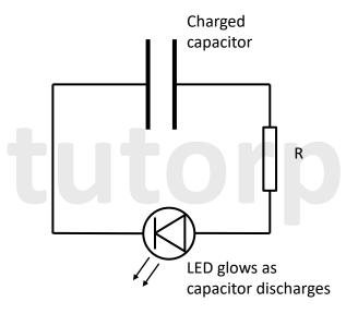
Consider capacitors as buckets that hold electrical charge. You can fill up the bucket and empty it when you feel like it. The capacitance of a capacitor tells you how much charge it can store.
