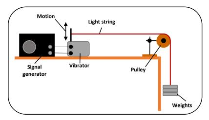
The above setup can be used to investigate the behaviour of vibrating strings. A string or wire is connected to the vibrator on one end. The vibrator is then connected to a signal generator. The other end of the string passes over a pulley and is supported by a weight, which keeps the tension in the spring constant.
