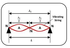
Therefore, the frequency of the 2<sup>nd</sup> harmonic vibrations is:
