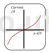
The temperature of the thermistor rises as the current through it increases. The decreasing resistance is indicated by the increasing gradient of this characteristic graph.
