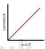
The current flowing through an **ohmic conductor** is proportional to the p.d. that pushes it. As a result, it follows Ohms law and so for this conductor V = IR.
