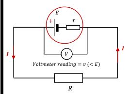
The circuit opposite shows a cell with an e.m.f. (E) and internal resistance r connected to an external resistor of resistance R. The current from the cell flows through its own internal resistance as well as the external resistance. As a result, the voltmeter reading is less than E.
