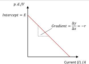
E.m.f. (E), terminal p.d. (V), current (I), and internal resistance (r) are linked by the following equation:
