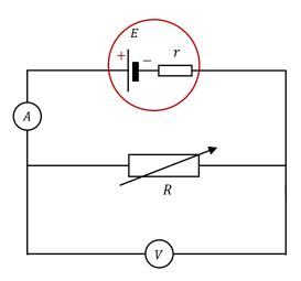
The circuit illustrated above is used to determine the e.m.f. (E) and internal resistance (r) of a cell with greater accuracy.
