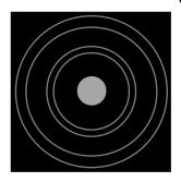
Diffraction is a wave phenomenon and since these electron diffraction rings are very similar to those obtained when light passes through small, circular aperture (light, dark, light, etc...), they provide strong evidence for the behaviour of matter proposed by de Broglie.
