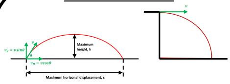
If an object is thrown in any direction it will follow a curved (or parabolic) path through the air. Acceleration due to gravity only acts on the object vertically downwards and the object has no horizontal acceleration.
