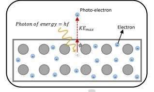
When a **photon of energy (hf)** causes photoemission from a metal surface, some of the photon energy is used to overcome the **work function** ( $\phi$ ), while the rest is released as kinetic energy.
