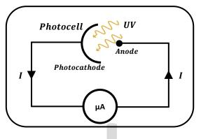
The photoelectric current, as measured by the microammeter, is proportional to the number of electrons flowing between the cathode and anode per second. Therefore, a high microammeter value indicates a high number of electrons released per second.
