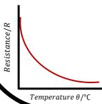
Negative Temperature Coefficient (NTC) Thermistor Graph: over a narrow range of temperature, resistance drops rapidly.
