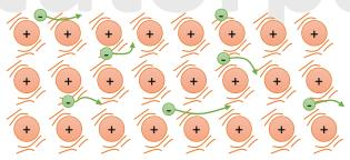
Hence, the electron—ion collisions are more frequent, slowing the flow of electrons (i.e. the current is reduced).
