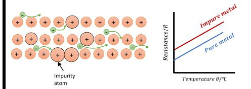
Because the impurity atoms and metal ions are of different sizes, the frequency of collisions experienced by the drifting electrons increases.
