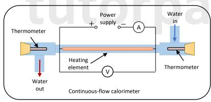
• Re-do the experiment, adjusting only the power supply's p.d. and the flow rate (mass) so  $\Delta\theta$  remains constant. For each experiment, you should now have an equation:
