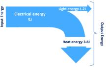
A light-emitting diode (LED) is supplied with 5 J of electrical energy each second, and produces 1.2 J of light and 3.8 J of heat energy. What is its efficiency?
