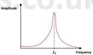
Resonance occurs when the **forcing frequency is equal to the natural frequency** of the system and the **maximum amplitude** is achieved. The frequency at which it occurs is called the resonant frequency.
