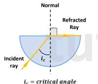
If the angle of incidence is increased to a particular value known as the **critical angle**, the light ray refracts along the boundary.
