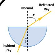
When light rays pass through glass and into air, they refract away from the normal.
