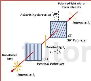
$I_0$  is the unpolarised light's initial intensity before going through the first vertical polariser.
